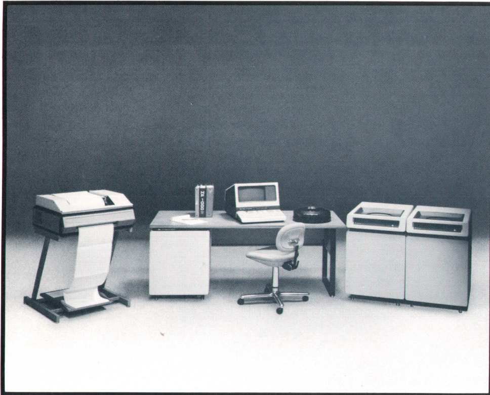
Fig. 1. The new Model 45, the most powerful HP 1000 System, features the new F-Series Computer with floating-point processor and the new RTE-IV operating system. It is designed for applications involving extensive computation, large programs, large data arrays, and graphics. It is shown here with 100M bytes of disc storage.
