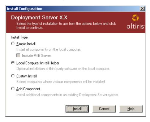
3. Select **Simple Install**, select the **Include PXE Server** checkbox, and then click **Install** to begin the installation process
