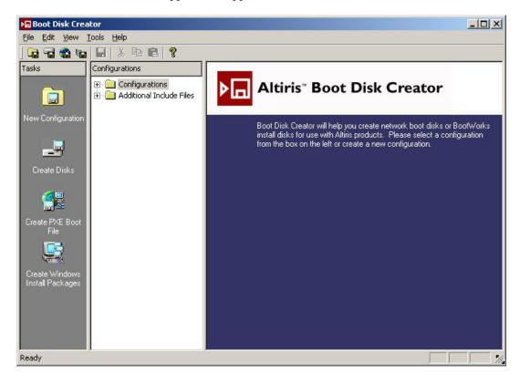
2. Click the **New Configuration** icon in the Tasks pane on the left. Enter a name for the configuration, such as DOS Boot Disk, and a description in the window that appears, and then click **Next.**
