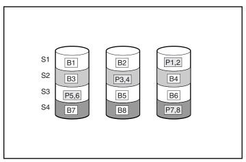
Figure A-7: Distributed data guarding, showing parity information (Px,y)
