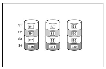
Figure A-3: Data striping (S1-S4) of data blocks B1-B12
