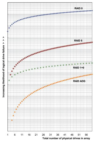
Figure B-1: Relative probability of logical drive failure
