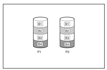
Figure A-5: Drive mirroring of P1 to P2
