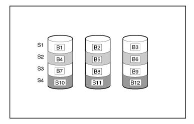
For data in the logical drive to be readable, the data block sequence must be the same in every stripe. This sequencing process is performed by the array controller, which sends the data blocks to the drive write heads in the correct order.
