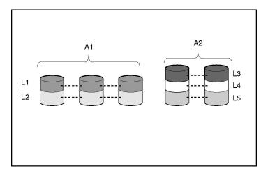
Each logical drive in an array is distributed across all of the physical drives within the array. A logical drive can also extend across more than one port on the same controller, but it cannot extend across more than one controller.
