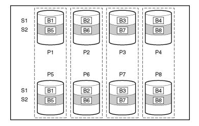
In each mirrored pair, the physical drive that is not busy answering other requests answers any read requests that are sent to the array. (This behavior is called **load balancing.**) If a physical drive fails, the remaining drive in the mirrored pair can still provide all the necessary data. Several drives in the array can fail without incurring data loss, as long as no two failed drives belong to the same mirrored pair.
