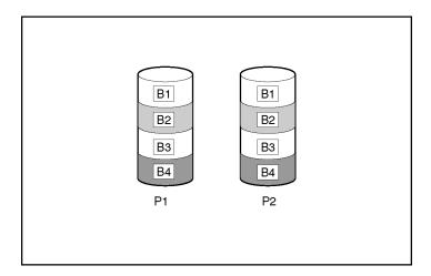
When the array has more than two physical drives, drives are mirrored in pairs.
