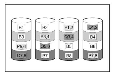
This method is most useful when data loss is unacceptable but cost is also an important factor. The probability that data loss will occur when an array is configured with RAID ADG is less than it would be if it were configured with RAID 5.
