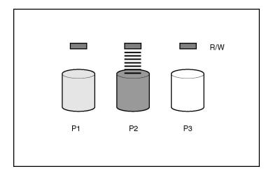
With an array controller installed in the system, the capacity of several physical drives can be combined into one or more virtual units called **logical drives** (also called **logical volumes** and denoted by Ln in the figures in this section). Then, the read/write heads of all the constituent physical drives are active simultaneously, reducing the total time required for data transfer.
