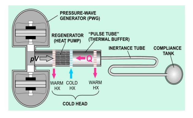
Figure 3: Thermoacoustic (pulse tube) Diagram
