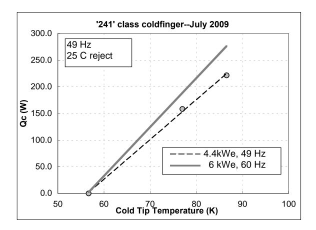
Figure 4: Approximate Cooling Load Curve with Rigid Transfer Line
