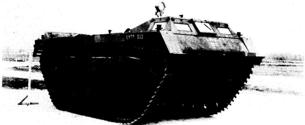
Figure 4-25. Landing Vehicle, Tracked, Mark III—1945 (APG A23239A) (Armament, 1 cal. .50, 2 cal. .30 machine guns. Armor, \frac{1}{2} " max., \frac{1}{4} " min. Crew, 2 to 7. Cruising range, 150 miles on land, 75 miles on water. Land speed, 21 mph. Net weight, 30,600 lb. Ground clearance, 19 in., Ground pressure, 8.75 psi. Dimensions: Length, 294 in., Width, 134 in., Height, 119 in.)
