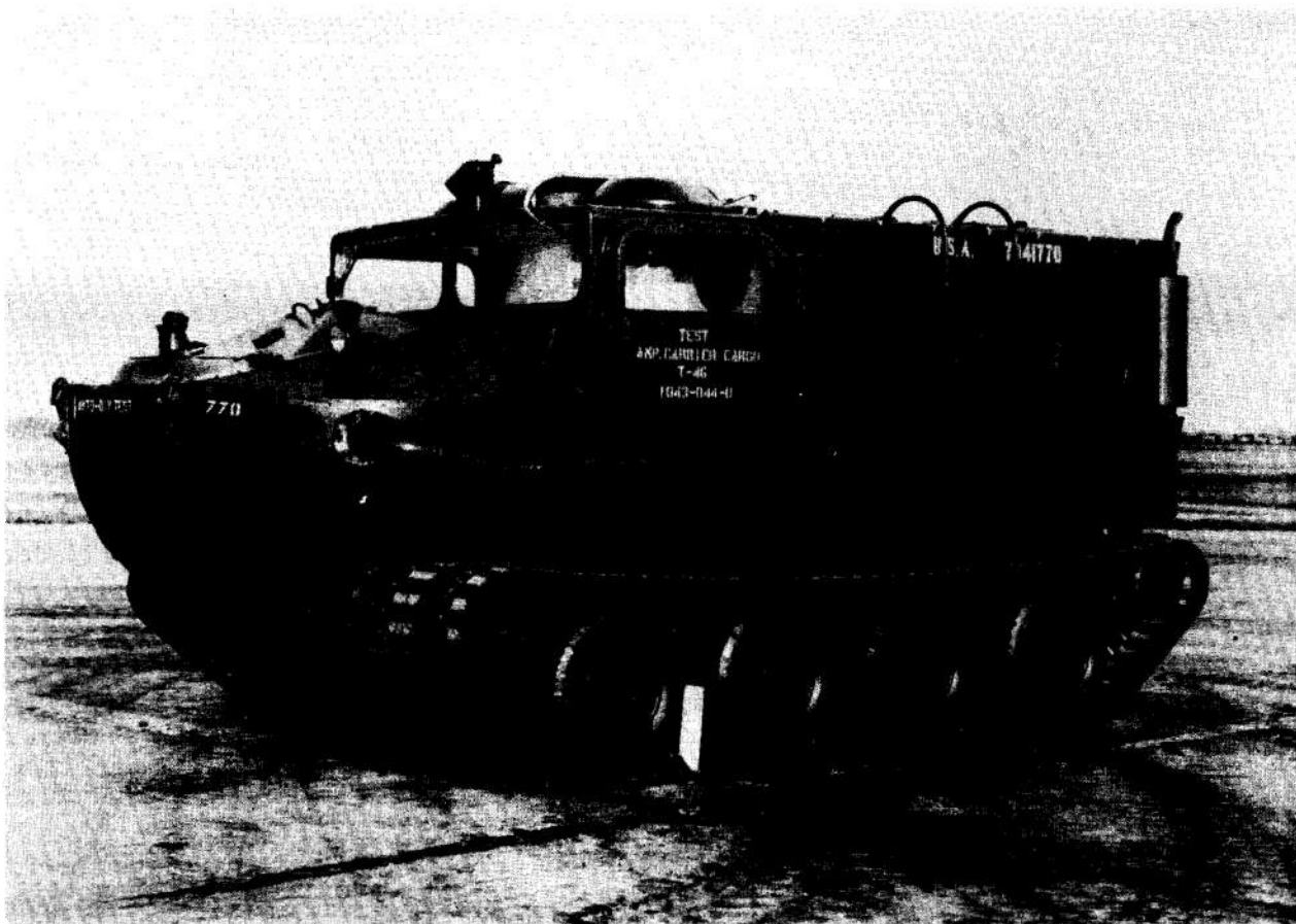
Figure 4-26. Amphibious Cargo Carrier, T46 (M76, Otter)—1949 (APG A59497) (Armament, cal. .50 machine gun. Combat weight, 12,162 lb. Ground pressure, 2.1 psi. Ground clearance 16- \frac{3}{4} in. Crosses trench 60 in. wide. Climbs obstacle 18 in. high. Max. gradeability, 60%. Cruising range, on land 140 miles, on water 5 hrs. Land speed, 28 mph. Dimensions: Length, 188 in., Width, 98 in., Height, 108 in.)
