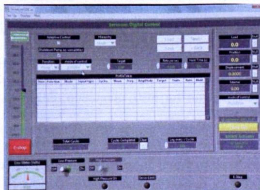
Figure 3.17 Display of Servocon loading controller
