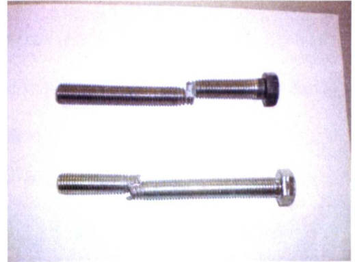
Figure B2 Bolt shank fracture after test
