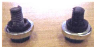
(b) Failure mode of bolt fracture
