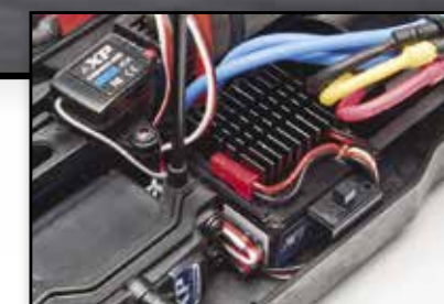
Water-resistant XP SC500-BL brushless speed control.
