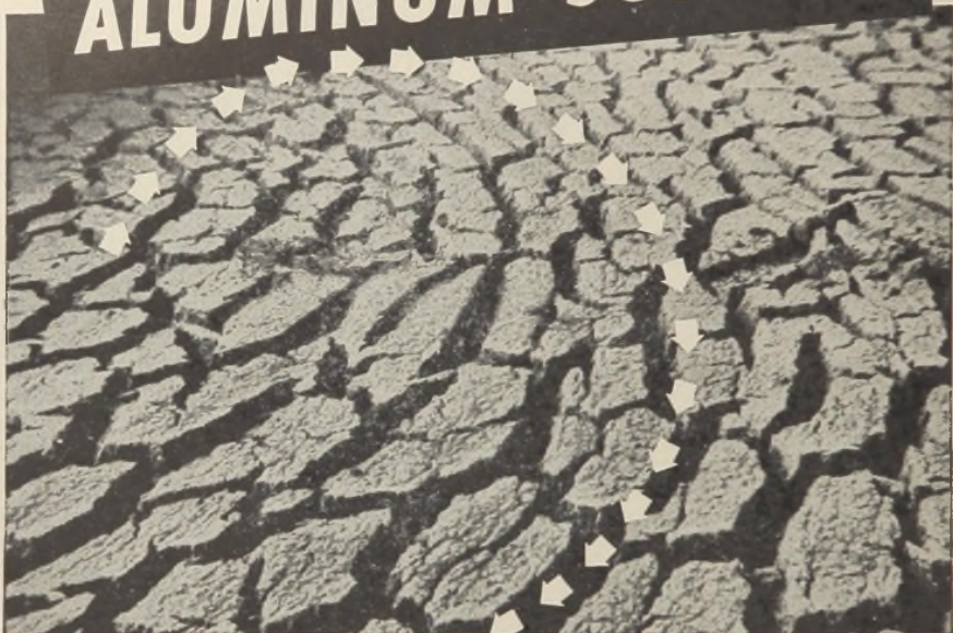
Well cracked sludge bed shortly after Aluminum Sulfate treatment.
