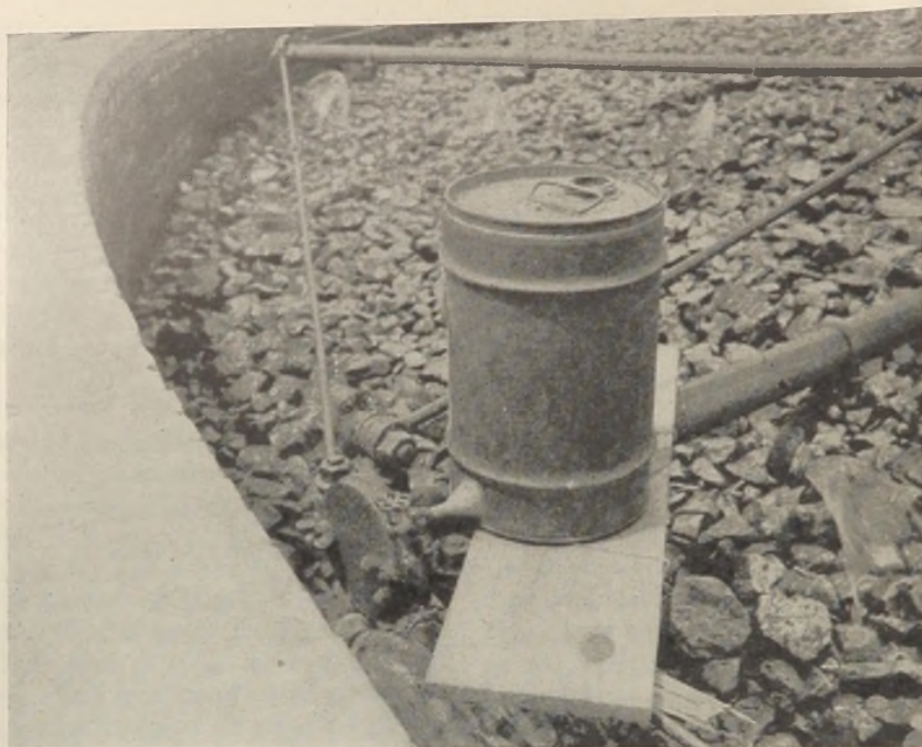
FIGURE 4.—Drip can mounted for feed of DDT emulsion in experiments involving selected areas.
