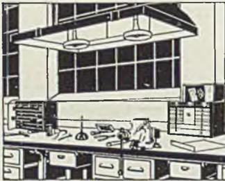
**Bench, Assembly and Inspection—**Where a high degree of diffusion is not required the Glassteel diffuser, the RLM dome reflectors equipped with white bowl lamps, or the deep bowl porcelain enameled reflectors will produce the desired result. Each job requires analysis to meet specific requirements. In some instances dual facilities must be provided, (1) diffuse lighting for certain defects, (2) directional lighting producing "glint" which may be essential to reveal others.
