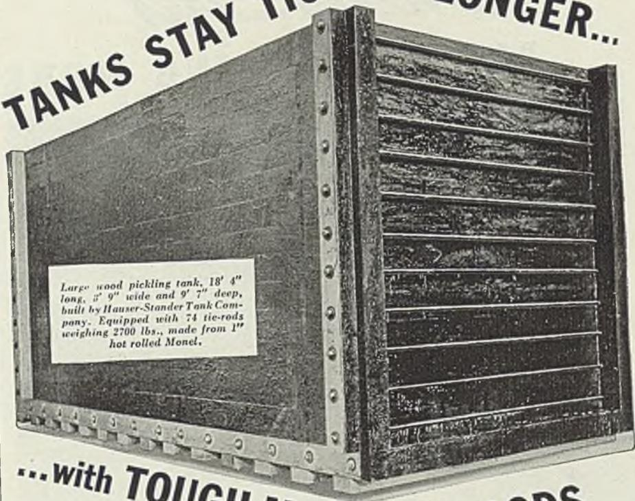
Large acid pickling tank, 18' 4" long, 5' 9" wide and 9' 7" deep, built by Hauser-Stander Tank Company. Equipped with 74 tie-rods weighing 2700 lbs., made from 1" hot rolled Monel.
