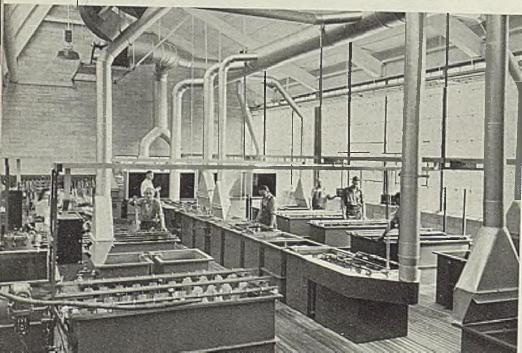
from other plating equipment here. This assures excellent working conditions and is an aid to maintaining the extremely high quality necessary on these parts.
