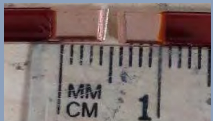
Figure 5. Trimmed Hairpins for Insulation Damage Limit Evaluation
