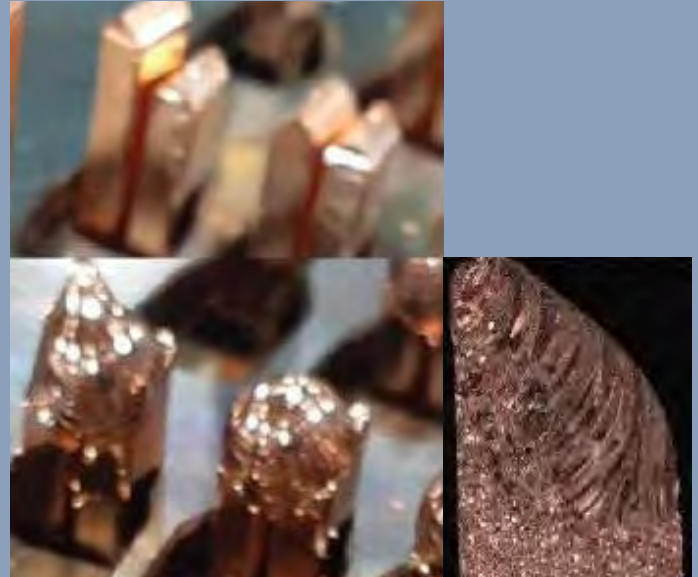
Figure 4. Before (top) and After (bottom) Hairpins Offset in Vertical Axis to Evaluate Process Tolerance
