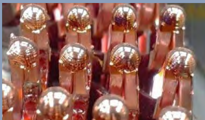
Figure 3. Multiple Hairpin Pairs EB welded on a Stator
