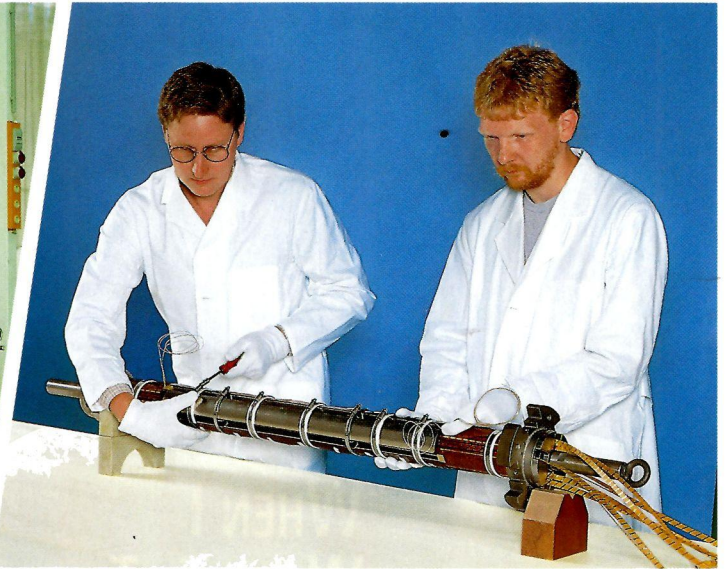
Assembly of the first short model coils of CQM magnets for the superconducting super collider SSC, USA
