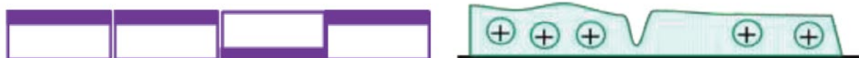
Figure 14: Sketches of wrong grain facets orientation (left) and oxides or other dielectric layers capable of charge accumulation, or ionic contamination spots (right).
