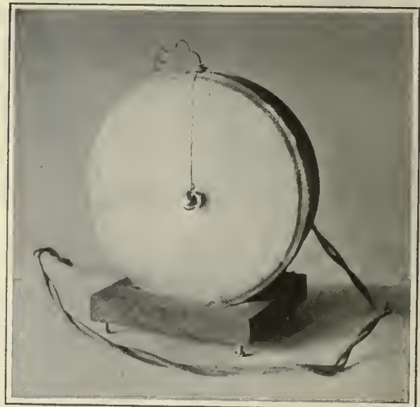
BERLINER'S FIRST MICROPHONE Of March 4, 1877. That illustrated is a replica made by him in 1879
