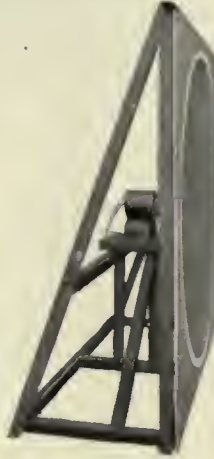
FIG. 5 A large cone speaker built in experimental form. Its mechanism is not unlike that of the Phonotron shown on the previous page. The cone of this model was about four feet in diameter
